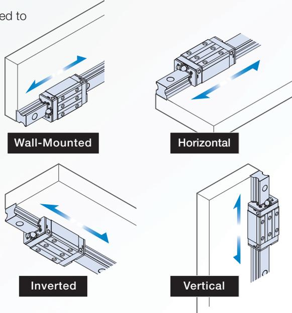
The Model HDR is equally suited for use in a horizontal orientation and any other orientation. The images are illustrative examples of LM Guide installations.
