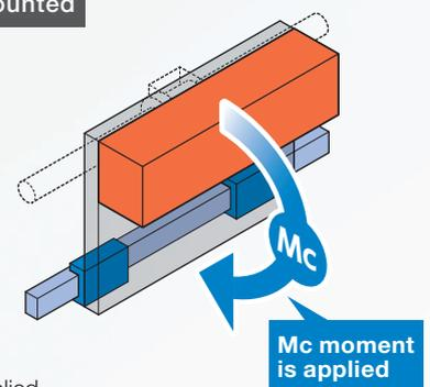
The Model HDR is ideal for applications where a constant  $M_c$  moment will be applied, such as configurations where an object will hang over the side of the table, or where the table is wall-mounted.
