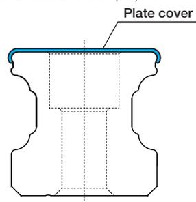
The plate cover placed over the entire upper surface of the LM rail greatly improves seal adhesion and helps prevent foreign materials from getting inside the LM block.
