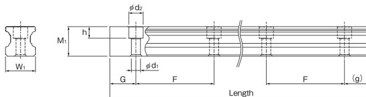
LM Rail Dimensions Unit: mm
